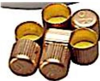
The percussion cap is a small metallic “cup” filled with a shock-sensitive primer, usually fulminate of mercury. The cap is placed on a pin in the rear of a gun barrel. When the pistol's hammer is released, it strikes the cap and ignites the primer which in turn ignites the gunpowder and fires the gun. This system replaced the flintlock arrangement which was prone to misfire. The percussion cap could also be used at the head of a grenade to set it off.
